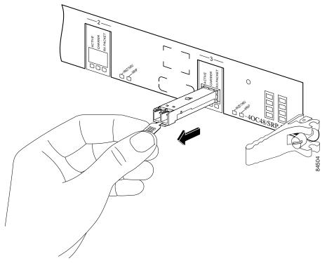
Step 4 Place the removed SFP module on an antistatic mat, or immediately place it in a static shielding bag if you plan to return it to the factory.
